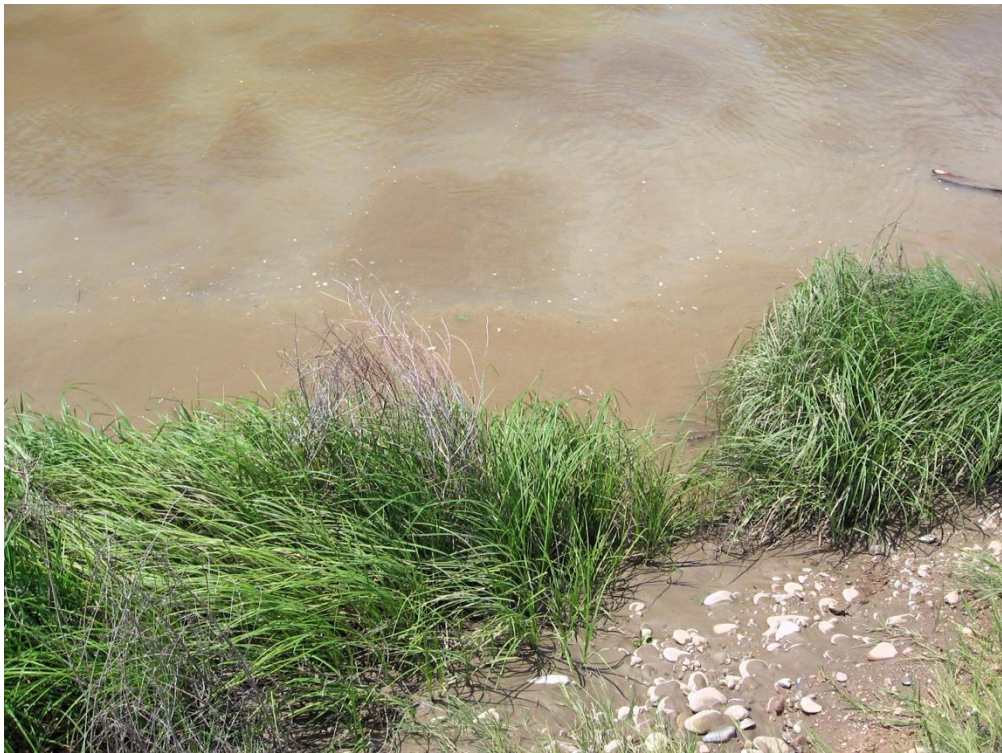
Point 13 minutes after application – 2:57 PM Water becoming clearer, flock pools more evident
