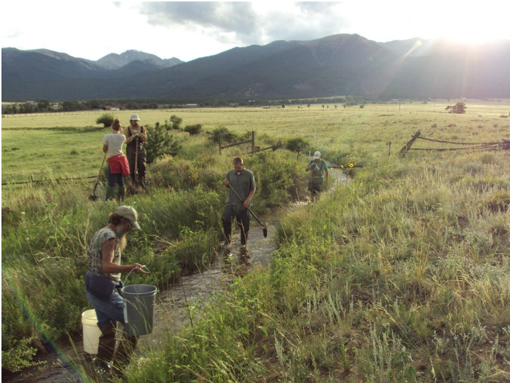
Soil being added to the Water to increase suspended solids
